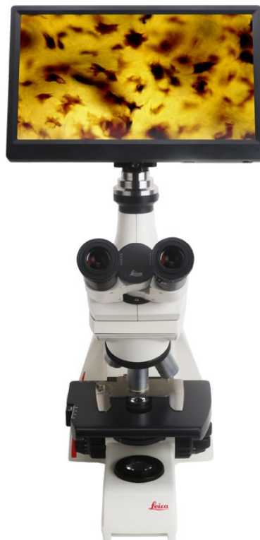
BLC-221 HDMI Camera on Leica Microscope
