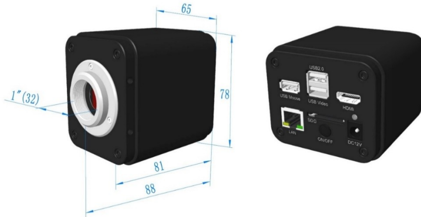
Dimension of BWHC2-4K Series Camera
