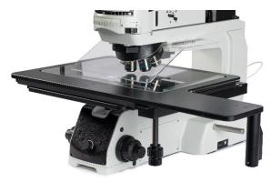
The focusing mechanism and fine adjustment handle of stage adopt the low hand position design, which conforms to the ergonomic design. Users no need to raise hands when operating, which gives the greatest degree of comfortable feeling.
