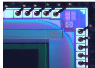
Bumping registration accuracy measuring in IC advanced package
