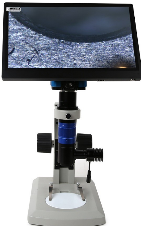
BS-1008-W100-TV050+BS-1008CL+ BS-1008SL(Coaxial Light Module)+ HDMI Camera
